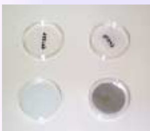
Clean and exposed filters.
