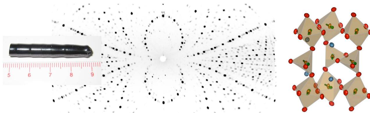
Figure 2. Our floating-zone grown crystal boule of  $\text{Ca}_2\text{Fe}_2\text{O}_5$  (scale bar is in cm) superimposed on a neutron Laue diffractogram (Koala) taken from the whole boule. The crystal and magnetic (canted AFM) structure on the right was refined against Koala data taken from a smaller fragment.
