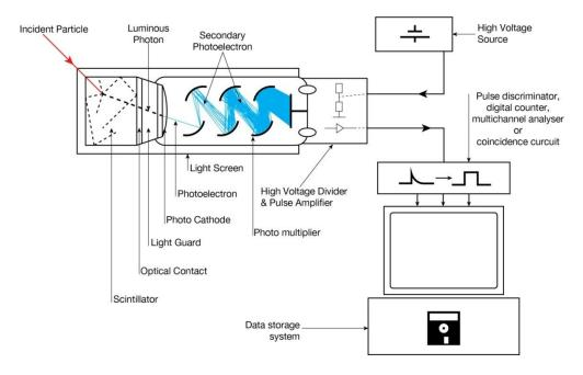
Schematic showing incident particles hitting a scintillating crystal, triggering the release of photons which are then converted into photoelectrons and multiplied in the photomultiplier. The photomultiplier can produce 10<sup>6</sup> electrons per photoelectron (Diagram source: Harry Mustoe-Playfair of Kings College London)
