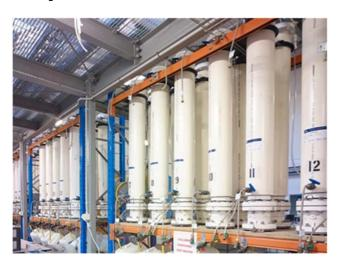
Some selected examples of large column leaching programs conducted to support PFS and DFS include the Ranger uranium mine, the Olympic Dam Operation and the Letlhakane Uranium Project. For the latter, integrated operation with a solvent extraction mini-plant was also undertaken.
