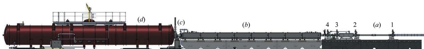
**Figure 1** An overview of the BILBY instrument. (a) The neutron guide, which starts at the reactor wall, and connecting choppers marked 1, 2, 3 and 4. For reference, the distance between choppers 1 and 2 is 4.4 m. (b) The ~17 m long collimator, (c) the sample area and (d) the 19 m long detector tank.
