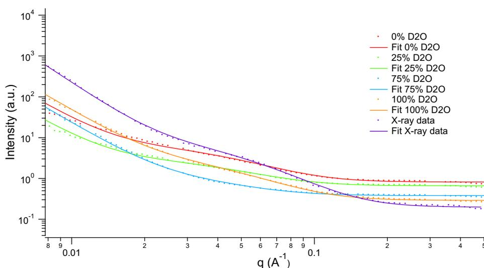
**Fig. 3.** SANS patterns of resistant starch formed from processed high-amylose maize starch in water. Four neutron solvent contrasts have been used: 0% D<sub>2</sub>O, (i.e. 100% H<sub>2</sub>O), 25% D<sub>2</sub>O:75% H<sub>2</sub>O, 75% D<sub>2</sub>O:25% H<sub>2</sub>O and 100% D<sub>2</sub>O along with an effective fifth contrast from SAXS. Dot points represent the experimental data that have been simultaneously fitted with a power law and two phase non-particulate model (solid lines).
