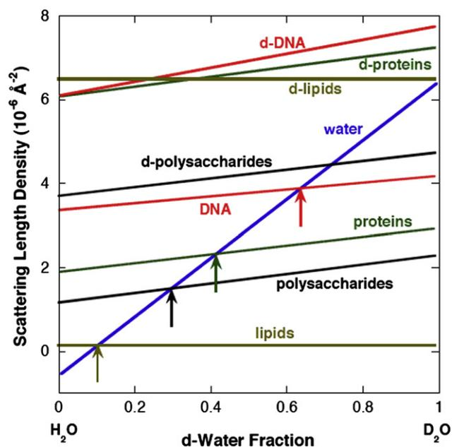
Fig. 2. Neutron scattering length densities for common food-based materials (with permission from Hammouda, 2008; adapted from Jacrot, 1976).
