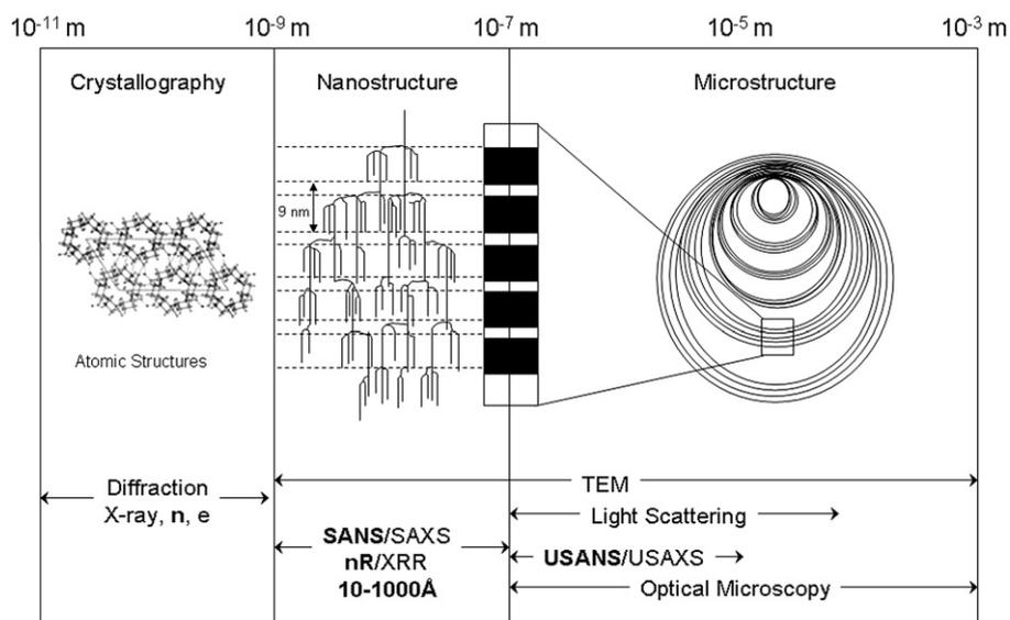
**Fig. 1.** The range of elastic neutron scattering techniques, corresponding size range and complementary methods shown in relation to the hierarchical structure of starch.
