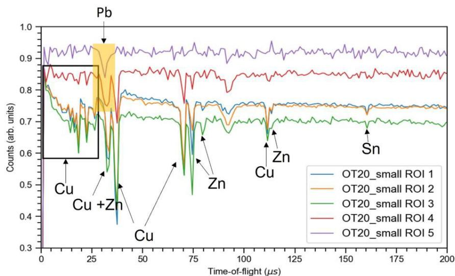
Figure 2. NRTI spectra (up to 200  $\mu\text{s}$ ) of the five ROIs selected for sample OT20. Peaks assignment is made in comparison with  $(n,\text{tot})$  cross section libraries<sup>3</sup> revealing the presence of copper, zinc, tin and lead. The full ToF range of NRTI spectra extends up to 2000  $\mu\text{s}$ .
