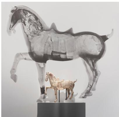
*Image: Figure of horse, ceramic, China, T'ang period, 618-906 CE. Powerhouse collection. Neutron radiograph by ANSTO*
