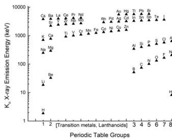
Fig. 1 – K $\alpha$  emission lines for the elements of the periodic table (data source: [11-12]).
