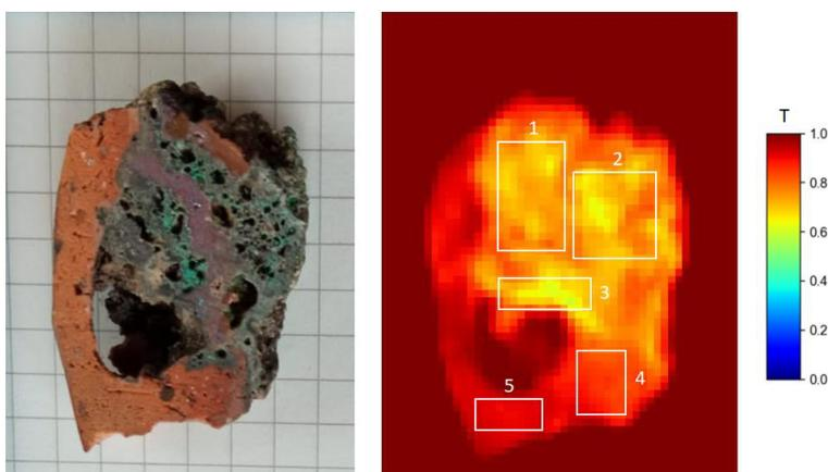
*Figure 1. On the left: crucible fragment OT20. On the right: the NRTI transmission map of the fragment. Based on the different transmission level, five Region Of Interest (ROI) are selected in order to determine their composition.*
