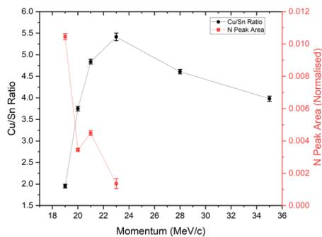
Fig. 3 – Copper/Tin Ratio (black) and nitrogen peak area variation (Red). The peaks used for the data analysis are the 115.9 keV peak for Cu, the 159.8 keV peak for Sn and the 101.0 keV peak for N.
