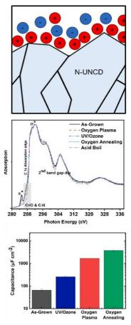
Nanocrystalline diamond in solution interacting with ions (top), Soft X-ray NEXAFS for carbon, illustrating the effect of different oxygen treatments (middle), and electrochemical cell capacitance measurements for different oxygen treatments (bottom)
