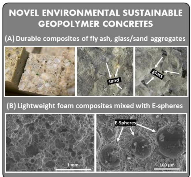
**Novel environmental sustainable geopolymer concrete materials** developed for enhanced durability (A) and lightweight property (B).
