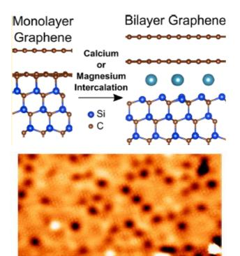
Scanning Tunnelling Microscope image of Ca intercalated on graphene
