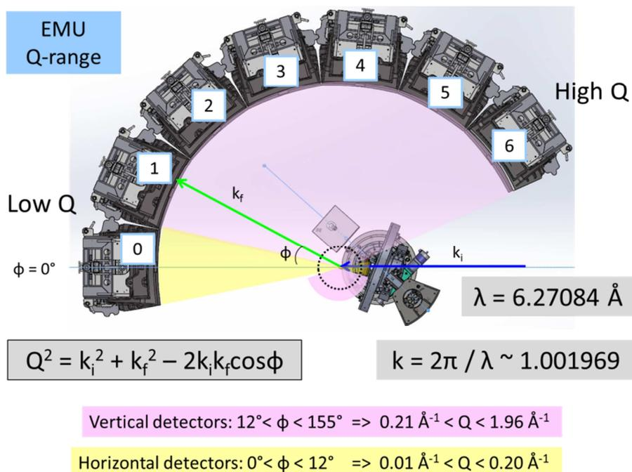
Figure 19. EMU Q-range calculated using  $k_i = k_f$ .
