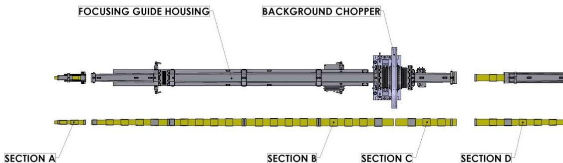
Figure 6: Focusing Guide with housing and the background chopper located between Sections B and C.
