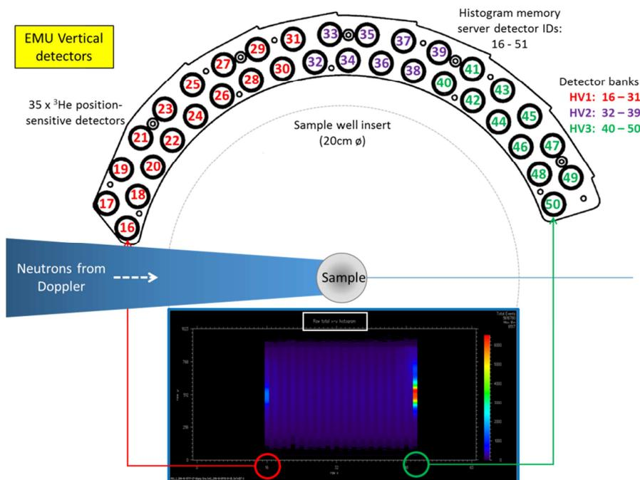
Figure 16: Stepwise configuration of the EMU vertical detectors, their HV connections and histogram memory server ID numbers.
