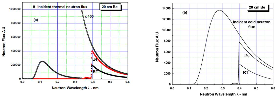
Figure 4. Transmitted neutron flux through polycrystalline beryllium. (Reproduced from [2]<sup>2</sup>)
