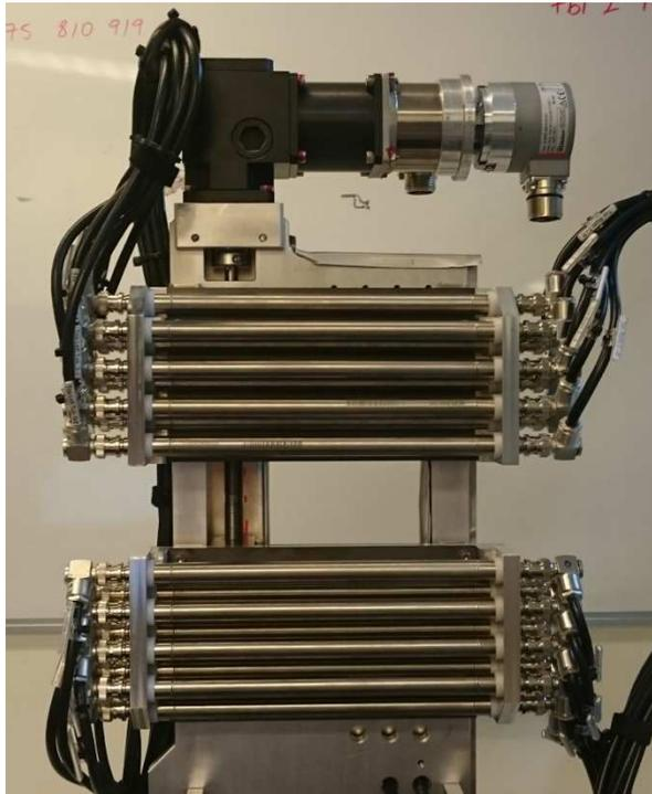
Figure 17: EMU horizontal detectors, mounted upon slits for beam size adjustment
