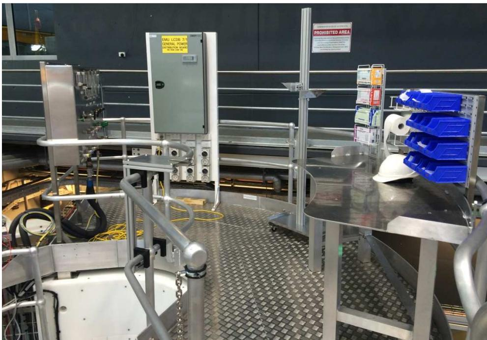
Figure 20. EMU Operating platform, sample preparation table and service panel
