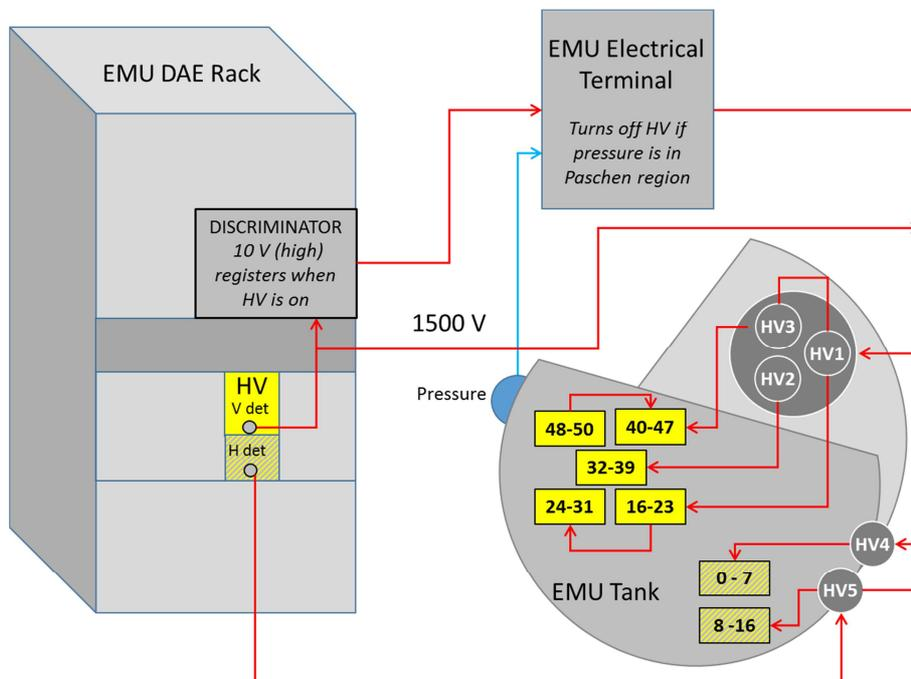
Figure 18: EMU detector connections to HV illustrating detector ID and HV connector.
