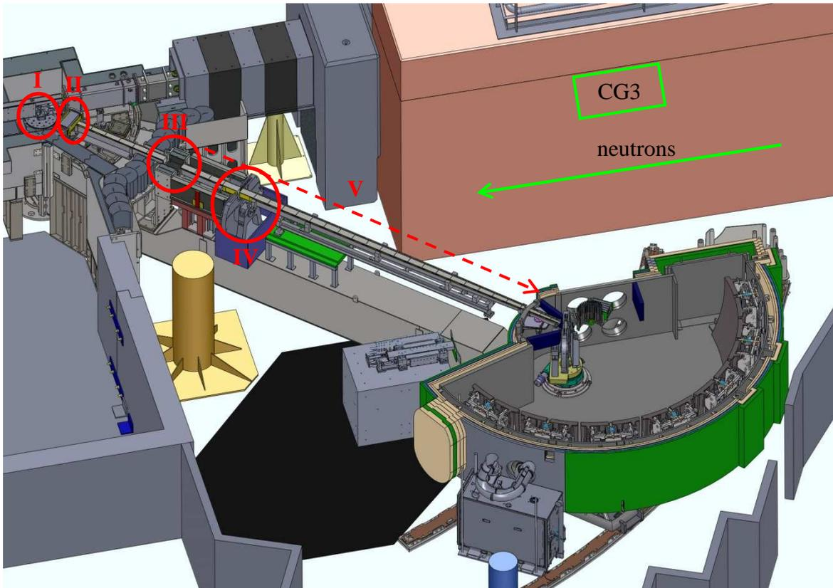
Figure 2: Conceptual design of the EMU spectrometer (side view)
