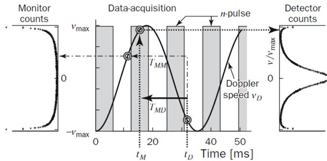
**Figure 12. Data acquisition on a reactor-BS instrument with Doppler monochromator. Neutrons which are counted at time  $t_D$  have been at the moving monochromator at time  $t_M = t_D - T_{MD}$ . The flight time  $T_{MD}$  is assumed to be constant. (Reproduced from ref [Error! Bookmark not defined.]**
