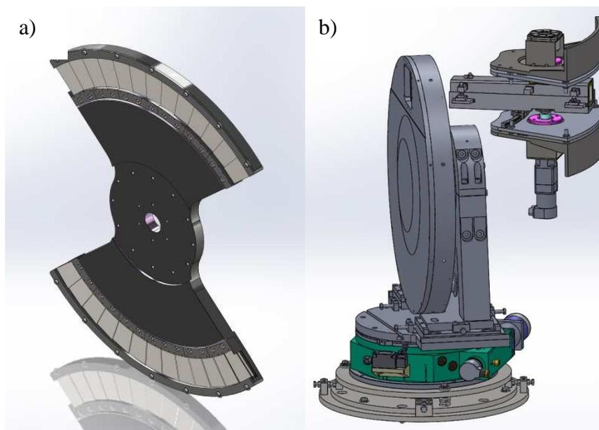
Figure 8: Graphite chopper a) disc (showing mounted crystals) and b) housing
