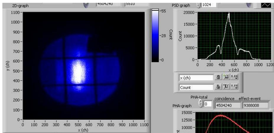
Figure 7. EMU beam profile at exit of focusing guide. Image obtained in air using a neutron camera.
