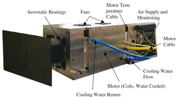
Figure 11: Doppler drive unit with a test backscattering monochromator support
