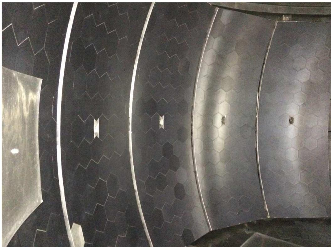
Figure 14: Analyser arrays fitted inside the scattering tank
