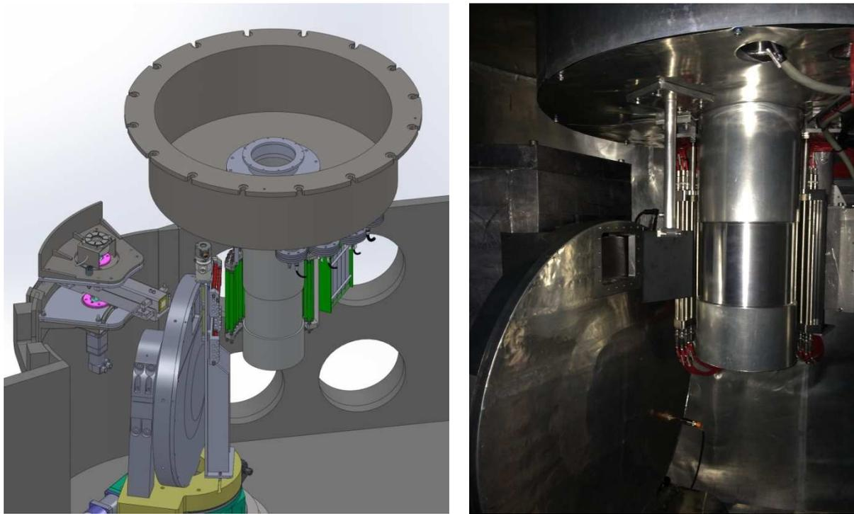
Figure 15: Vertical (green) and horizontal (red) detector arrays in place on the sample well and next to the graphite chopper, respectively.
