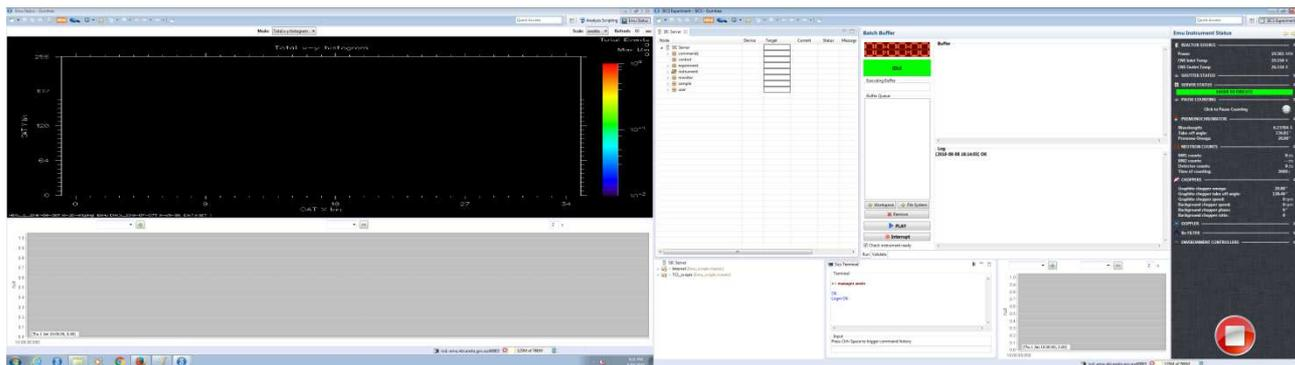
The black panel on the right side of this window is the **Gumtree dashboard** providing an overview of the current status of the reactor source and the current configuration of EMU instrument components (Premonochromator, Graphite chopper, Beam monitors, Doppler Drive, Environment Controllers).
