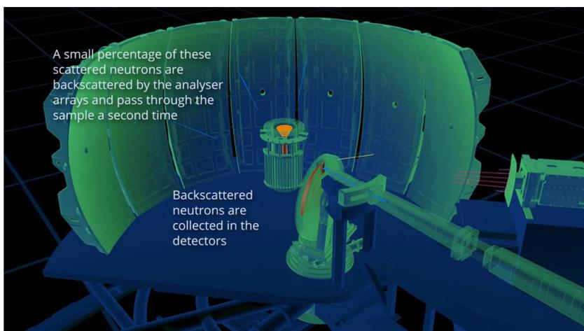
Figure 21. ANSTO YouTube video of EMU – simulating the neutron path through the instrument
