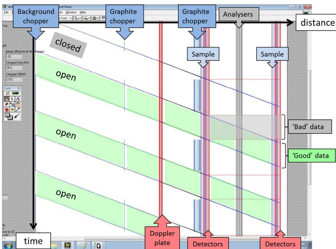
Figure 9. Time-distance diagram for EMU showing all major components of instrument.
