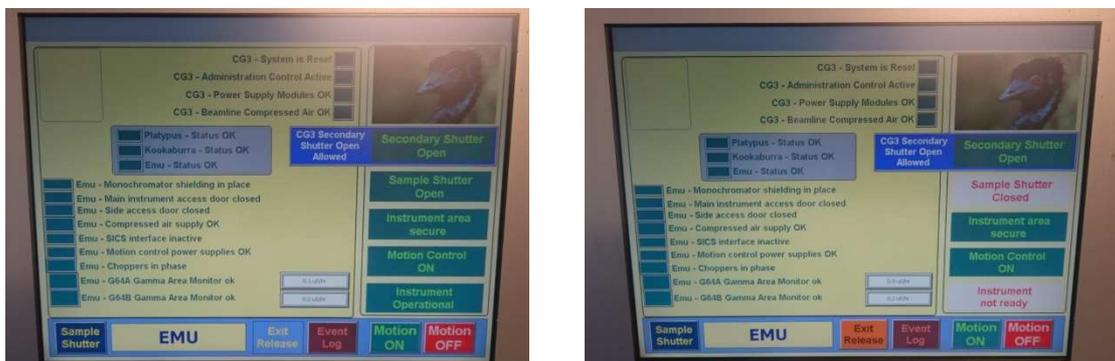
Figure 23: EMU Safety Control Panel. Green boxes indicate shutter is open (left). Orange 'Exit Release' button located bottom of screen (right).
