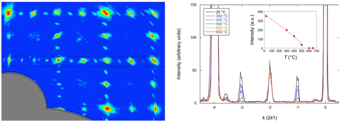
Figure 1. (Left) Reconstructed precession image of the zeroth-order Laue zone of  $\text{Sr}_2\text{Fe}_2\text{O}_5$  from Wombat data at room temperature. (Right) Integrated intensities along the line indicated by the black box on the left-hand figure, showing the disappearance of the superstructure peaks at  $540\text{ }^\circ\text{C}$ .
