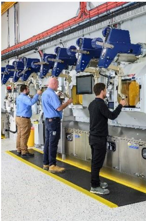
Above: Producing Mo-99 at the Mo-99 Manufacturing Facility using hot cells and arm manipulators
