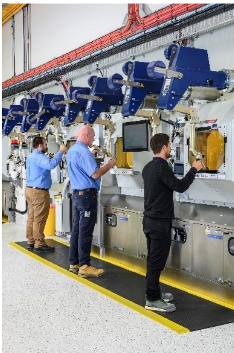
Above: Producing Mo-99 using hot cells and arm manipulators
