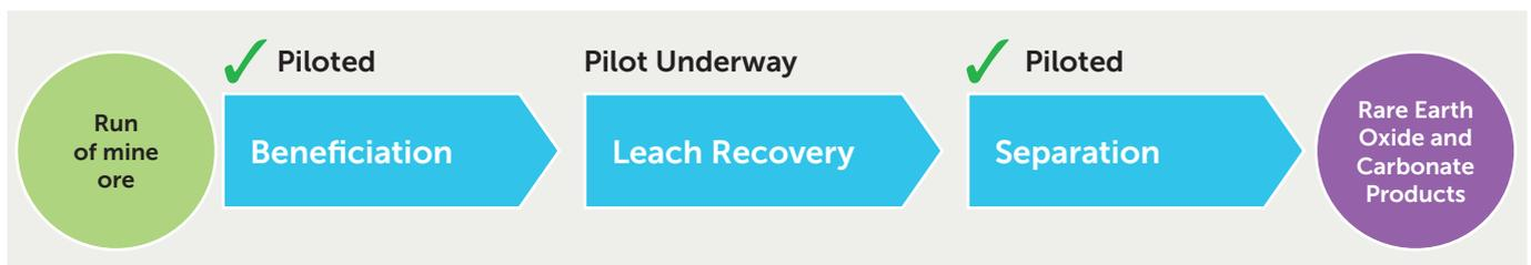
**Figure 1:** Three stage process developed by Peak for Ngualla's rare earth mineralisation and pilot plant status.
