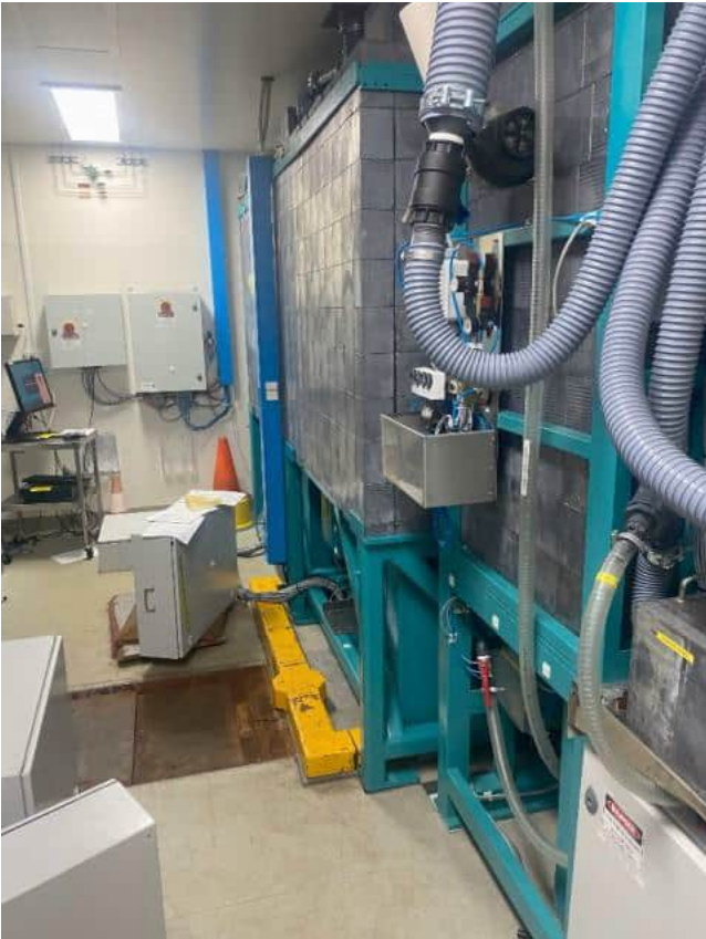
Photograph 17: Process unit on ground floor. Lead bricks are used around the unit. Photo direction: Not applicable
