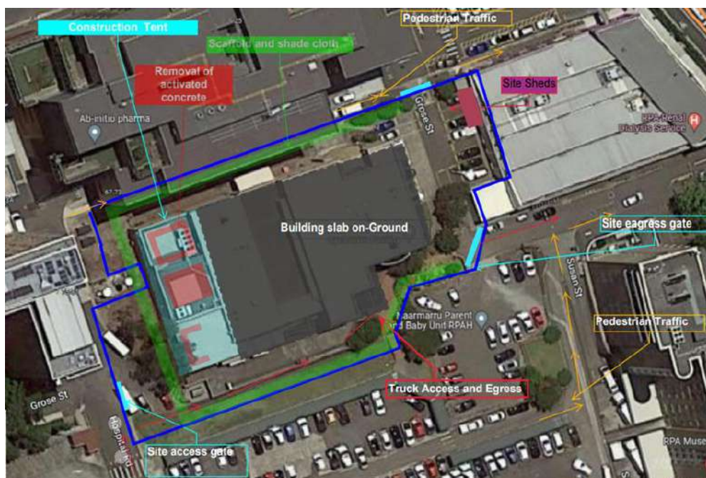
Figure 18 Image of Proposed Truck Access and Egress During D&D Activities
