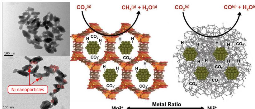
Electron microscopy (left) shows the formation of Ni nanoparticles following thermal annealing of NiMg-MOF-74. The resultant hybrid material facilitates catalytic conversion of CO<sub>2</sub> to either methane or carbon monoxide, depending on the Ni to Mg ratio in the original MOF (right).
