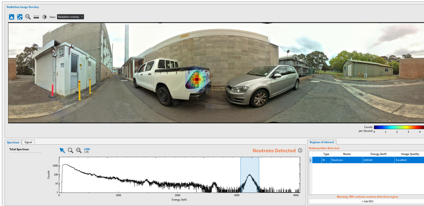
Case Study 1: CORIS360 ® GNI rapidly detected and localized thermal neutrons from a moderated 9 MBq (243 \mu Ci) neutron source hidden within a parked vehicle. CORIS360 ® GNI was at a standoff distance of 4 metres (13 feet) from the vehicle and imaged the neutron source in <15 minutes.
