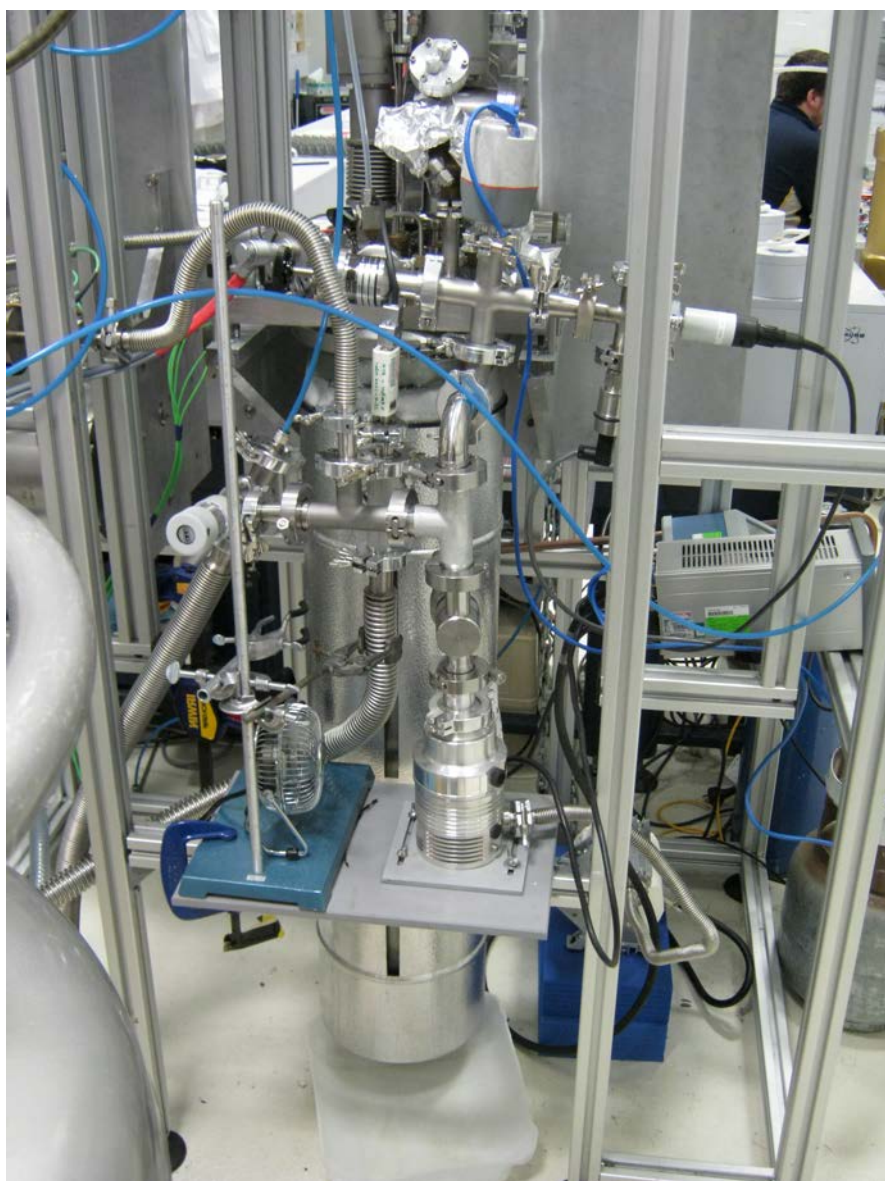
Figure 2 The Enclosive Flow Cooling (EFC) Cell; designed & built by S. Baurecker. Permanently on loan to the Australian Synchrotron from the Molecular Spectroscopy & Centre for Biospectroscopygroup at Monash University, Clayton. EFC may be run at liquid Helium Temperatures.
