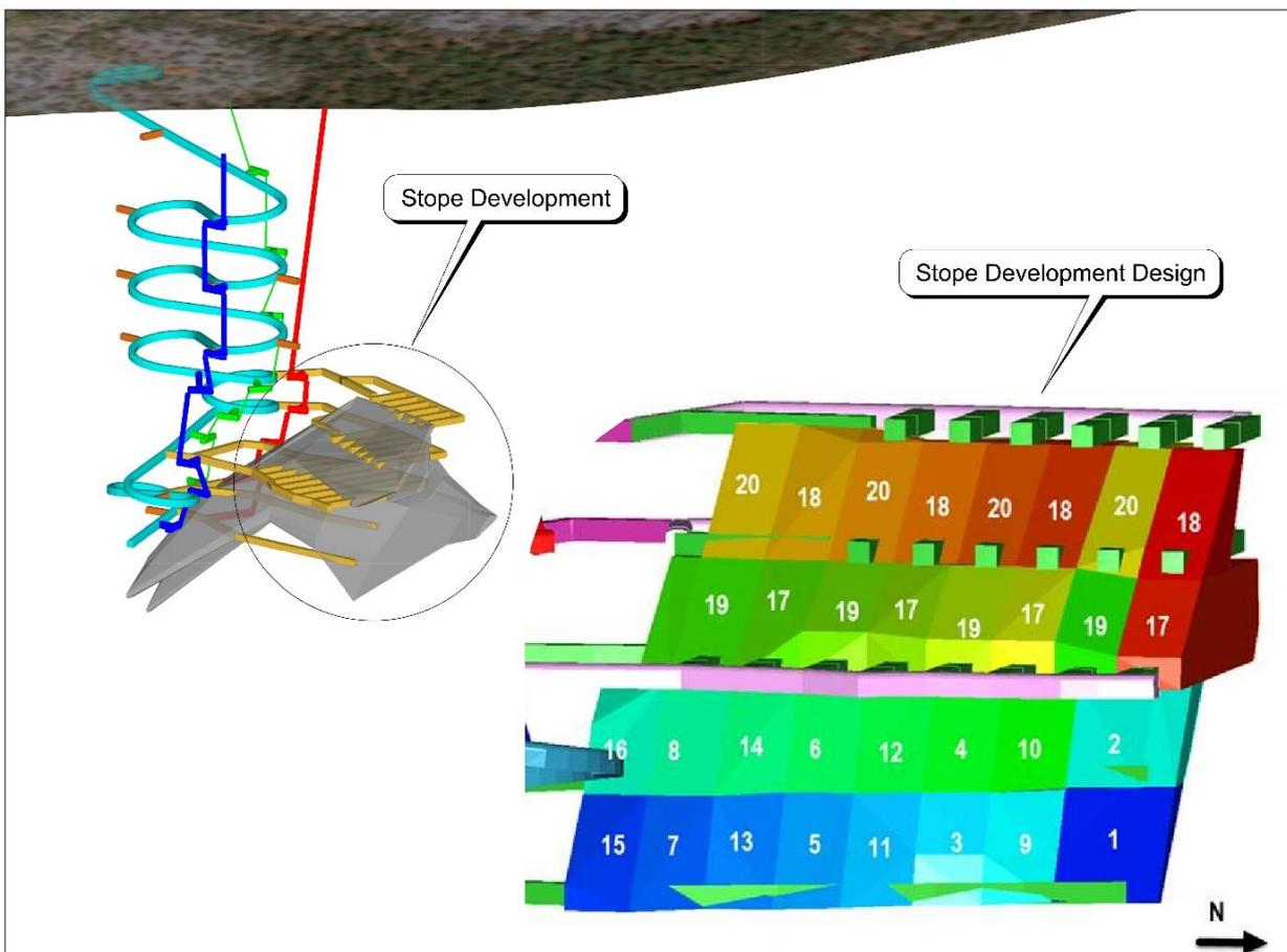
Figure 1: Angularli mine design and stope sequencing
