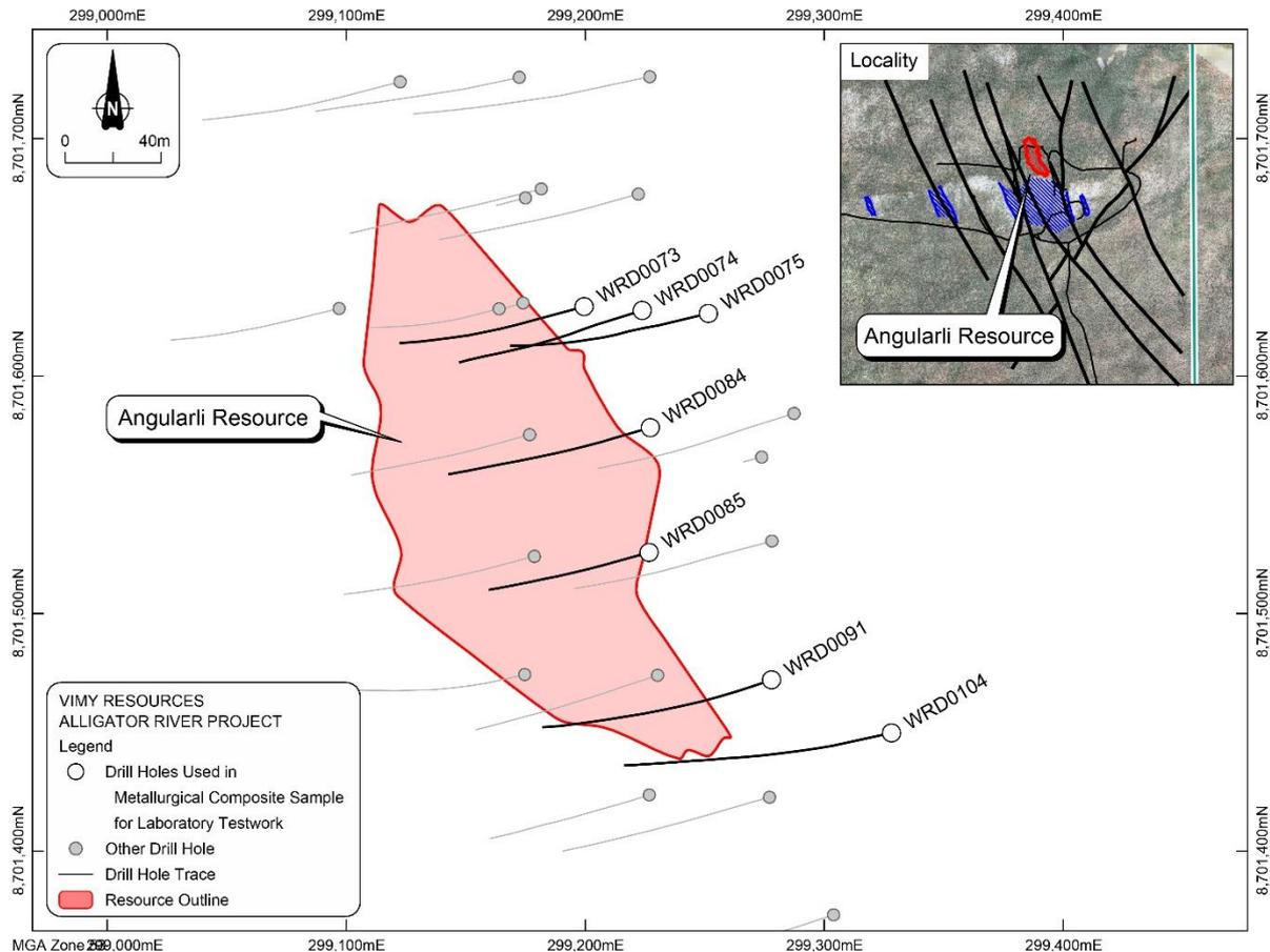
**Figure 2: Location of diamond drill collars used for metallurgical composite sample**
