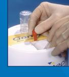
Grip the red protective cap (male luer closure), turn it anti-clockwise through 90° and remove from the outlet filter. With the sterile needle cover in place, attach a sterile needle (screw clockwise). Caution, do not over-tighten. Remove the sterile needle
