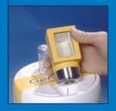
Observe the emptying of the saline vial and the filling of the evacuated elution vial, indicated by the sight and sound of air bubbles in the elution vial.
