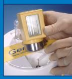
Place the needle cover back on to the sterile needle and leave it in place until the next elution. (Replace with a fresh sterile needle before each elution).
