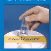
from the elution vial shield Unscrew the metal top. Remove the red flip-off seal from a 30 mL evacuated elution vial. Place the decapped vial in the elution vial shield and screw on the metal cap to hold the vial in place. Swab the top of the evacuated elution vial shield and the exposed part of the septum of the evacuated elution vial, with
