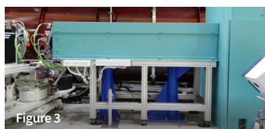
Figure 1. Image of the neutron beam line prompt gamma emissions that were causing dose rates above acceptable limits.
