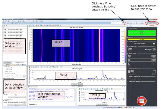
At the top left is the 'data source' window. You should add datafiles to this window by clicking on the green 'plus' icon. Note that only files that are in this window *and selected* will be processed. Underneath the data source window is the data reduction control window. You can select the type of data reduction by clicking on the 'Load Script' button and selecting from the list of recently used reduction scripts. See the individual sections below for the names of appropriate scripts to load.
