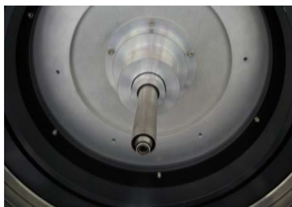
A view down the length of the Cobra nitrogen flow system directed into the detector drum on KOALA.
