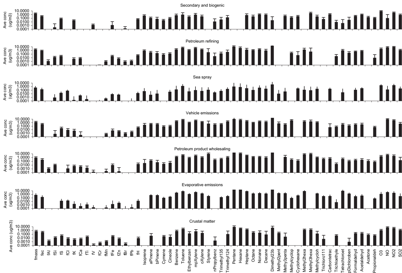
Fig. 4. Source profiles of fine particles, VOC and gaseous pollutants from PMF model analysis.
