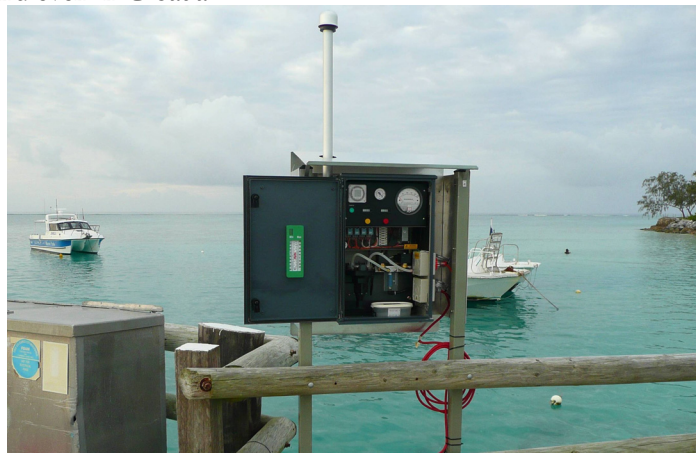
Fig. 1. ANSTO ASP sampling unit on Heron Island, Great Barrier Reef, Queensland, Australia.
