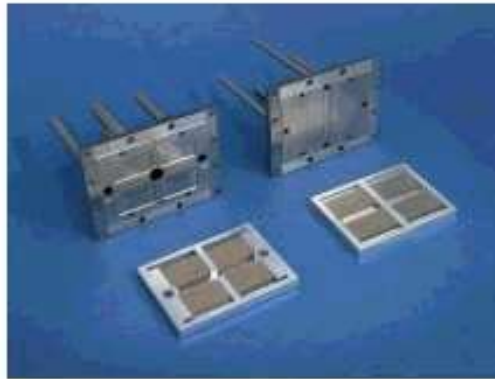
Batelle, Northwest National Laboratory Gasoline reformer
